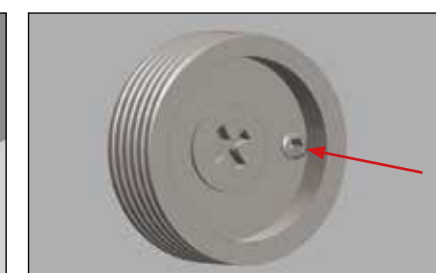
Secure with 3mm grub screw
