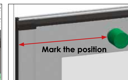
Mark the position with pencil
